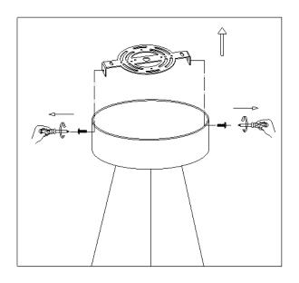
Step 1: Separate the bracket and fixture.
