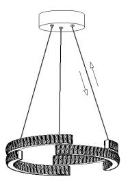
Step 5: Adjust the hanging wire, make the fixture level .
