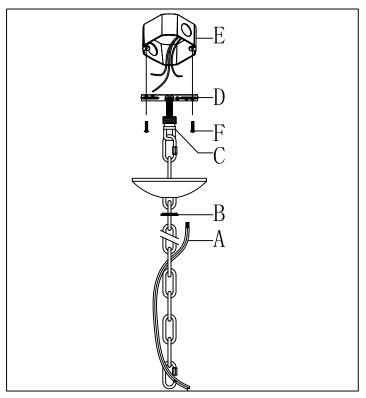
STEP 2:Wrap the Ground Wire from the fixture around the Green Ground Screw(G) on the Mounting Strap(D) and then connect the Ribbed Black Wire from the Fixture to the White Wire(Neutral wire) from the Outlet Box. Connect the Smooth Black Wire from the Fixture to the Black Wire(Live wire) from the Outlet Box. Cover the connections using the Wire Connectors(H). Slide Canopy(I) back up the Chain link and screw the Collar(B) back into place.
