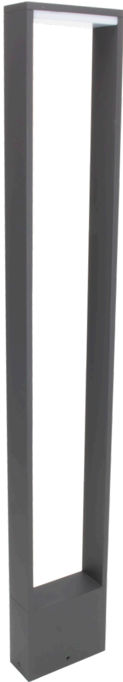
Stage Bollard Light BOL-STAGE-GT (120-277V / 10W / 450Lm) 5-15/16"W x 2-3/8"D x 39-13/32"H
